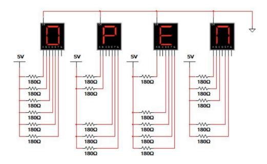
1. Using the CDS, enter this circuit and verify that it is working as expected (i.e., is OPEN being displayed?).
