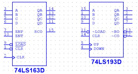
In short, the 74LS163 chip will use the ABCD inputs to define the starting points and endpoints of the counting, and the QA, QB, QC, and QD outputs to send a 4-bit binary number out to display. Similarly, the 74LS193 chip uses the ABCD inputs for the same definitions, the UP/DOWN inputs define the direction of counting, and the Q outputs give a 4-bit binary output for use in your circuit.
